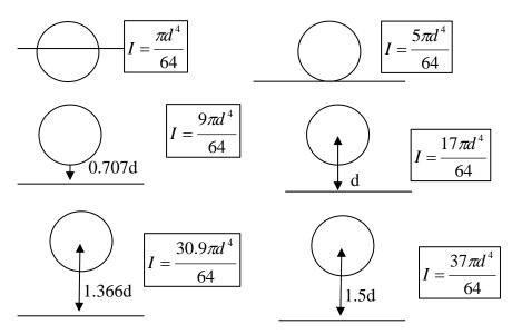
Where the straight line in each diagram is the axis of rotation. The first moment of area is for a circle about its centroid. The remaining I's are calculated using the parallel axis rule:
